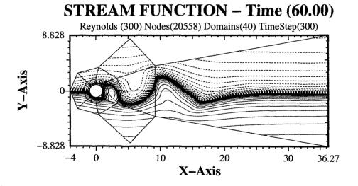
Figure 1 unsteady flow around a cylinder at Reynolds 300
