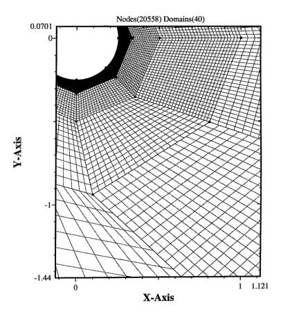
Figure 2 mesh used for computation of stream function and vorticity solutions
