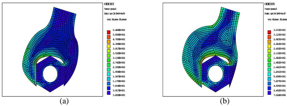
Figure 3: Initial and optimized shape of the spanner
