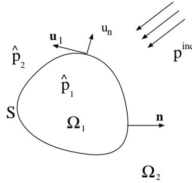
Figure 1: Structural-acoustic coupling
