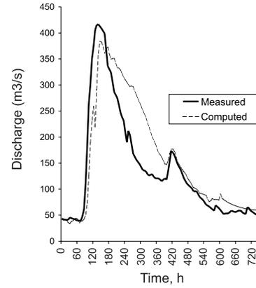
Fig. 5. Measured and computed hydrographs at the Gaviotas gauging station, May, 1970
