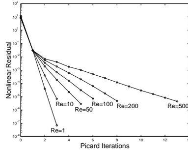
Figure 5.3: Convergence of Picard iteration for different Reynolds number
