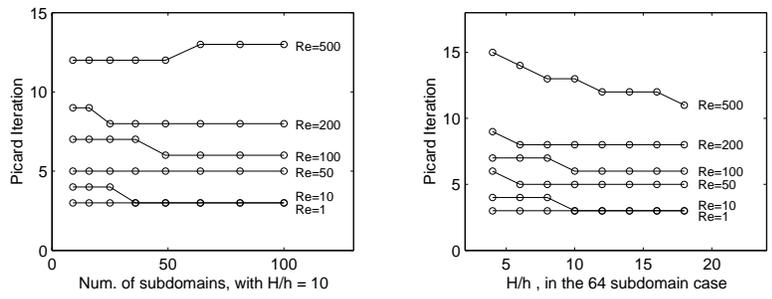
Figure 5.4: Convergence of Picard iteration for different meshes
