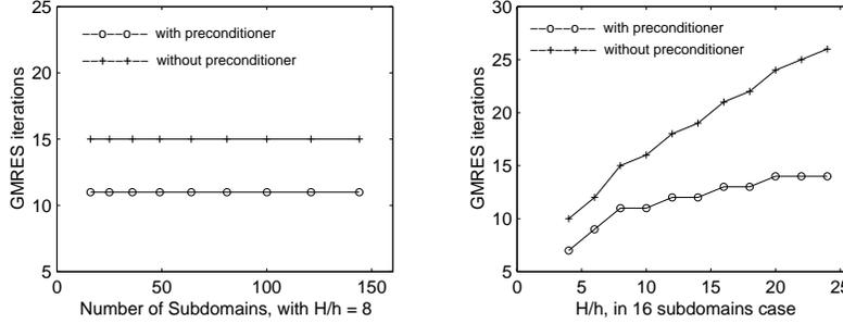
Figure 5.1: GMRES iterations counts for the Stokes solver vs. number of subdomains (left) and vs.  $H/h$  (right)
