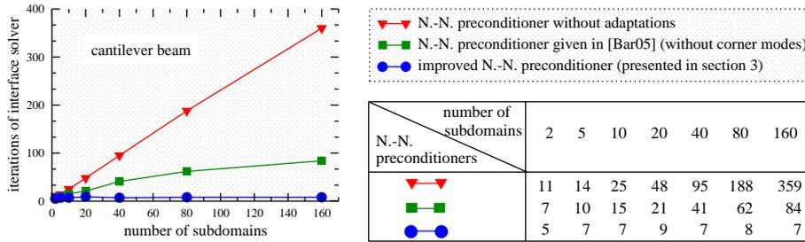
**Fig. 3.** Numerical scalability with Neumann-Neumann (N.-N.) preconditioners.
