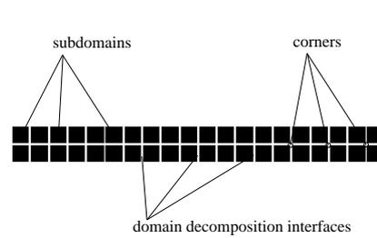
**Fig. 2.** Substructuring of the beam in 40 subdomains.
