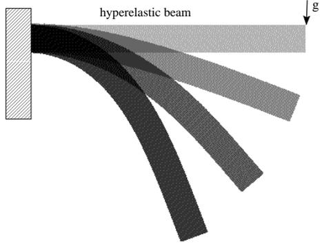
**Fig. 1.** Deformed sequence of a cantilever beam.
