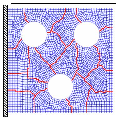
interface  $\Gamma$  shown in red partition nodes of  $\Gamma$  into corners, edges, faces
