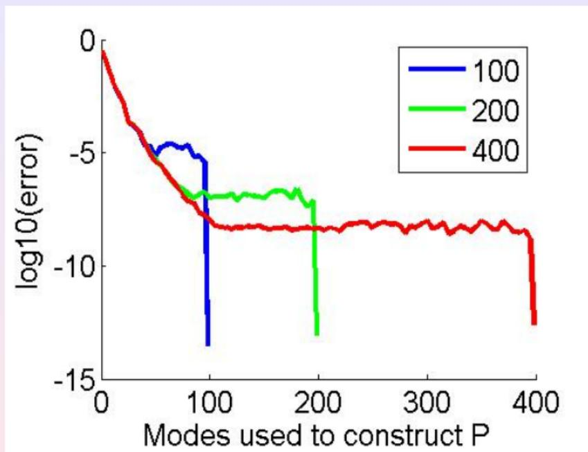
FIG.: influence of the approximation of the interface operator  $P_{[[\cdot, \cdot]]}$  on the convergence of the interface error
