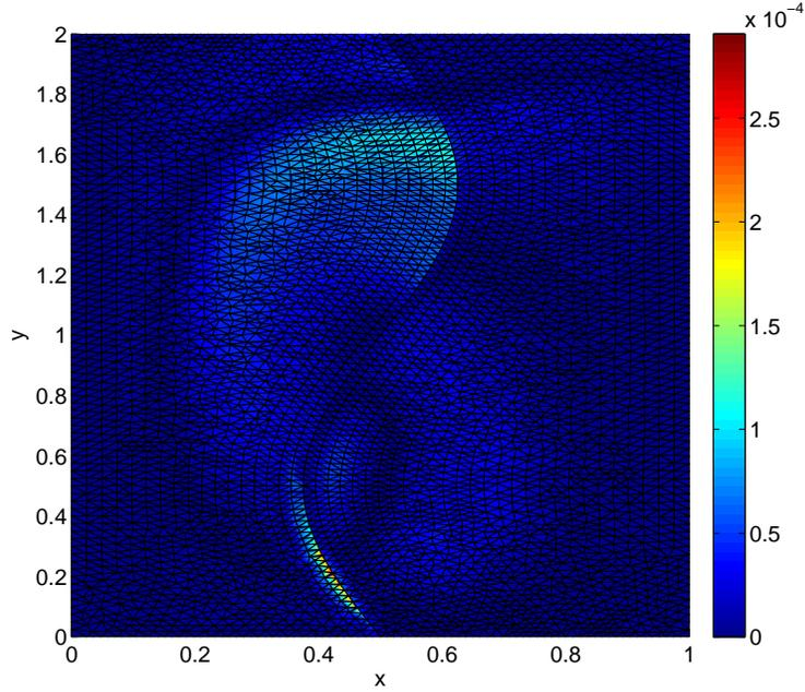
**Fig. 5.** Error between variational and DG-OSWR solutions, at final time, after 10 time windows and 3 iterations per window.
