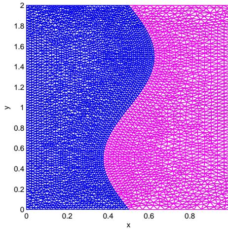
Fig. 4. Domain decomposition with  $\Omega_1$  (left) and  $\Omega_2$  (right).
