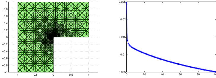
**Fig. 1.** *Left:* Refined mesh. *Right:* Gauss–Seidel convergence history.
