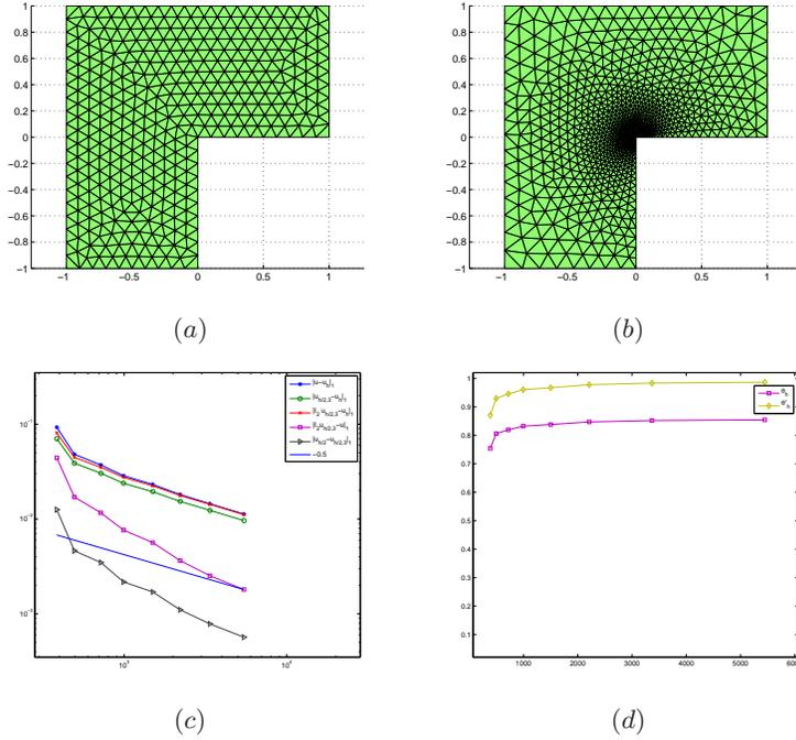
**Fig. 2.** Results of example 1. (a): initial mesh; (b): refined mesh after 4 refinements; (c): errors; (d): effectivity index.
