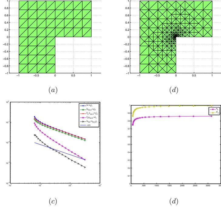
**Fig. 3.** Results of example 2. (a): initial mesh; (b): refined mesh after 8 refinements; (c): errors; (d): effectivity index.
