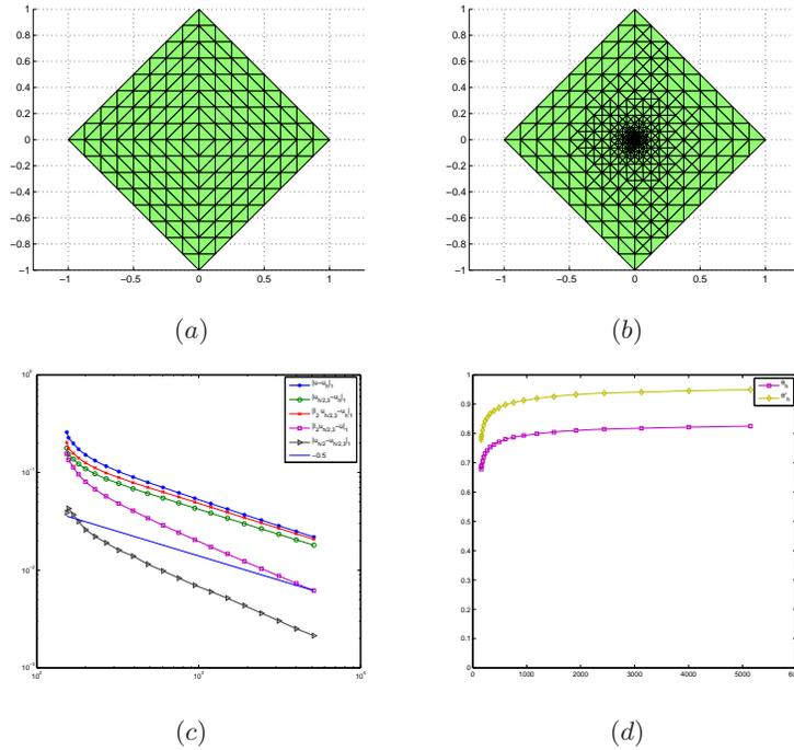
**Fig. 4.** Results of example 3. **(a):** initial mesh; **(b):** refined mesh after 8 refinements; **(c):** errors; **(d):** efficient index.
