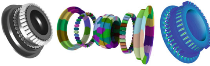
Fig. 3. Frictionless roller bearing of wind generator
