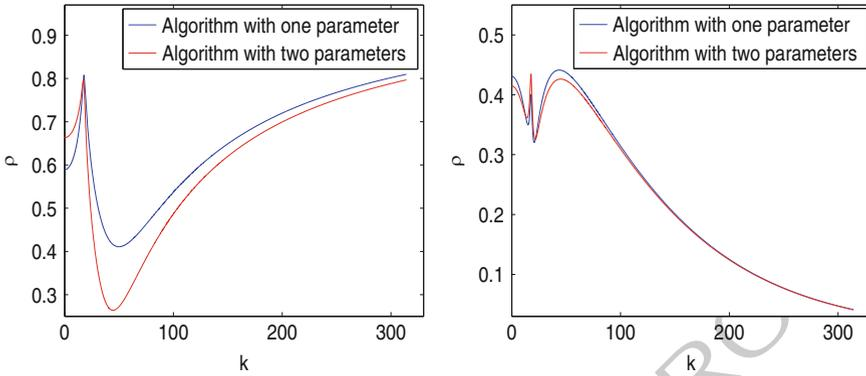
**Fig. 1.** Convergence factor comparison of algorithms with one and two parameters for  $\omega = 2\pi$ ,  $\sigma = 2$  and  $\mu = \varepsilon = 1$ , for the non-overlapping case,  $L = 0$ , on the *left*, and the overlapping case,  $L = h = \frac{1}{100}$ , on the *right*
