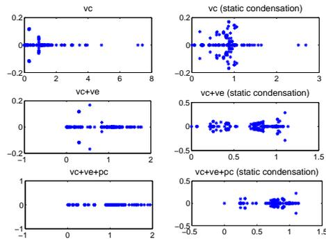
**Fig. 2** 3D Stokes problem: Eigenvalue distribution depending on the choice of primal unknowns and the static condensation, left column (without the static condensation) and right column (with the static condensation).
