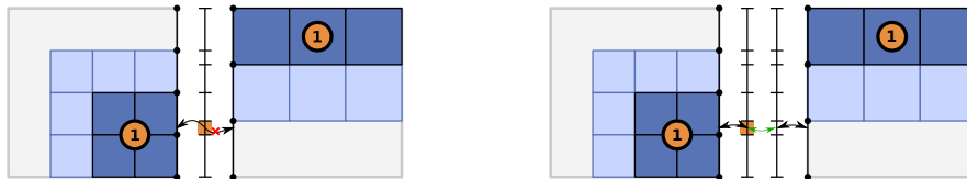
Fig. 4 Through the use of auxiliary spaces on the coupling interface \Gamma , direct access to non-local cells of the neighboring domain is avoided. (Numbers in circles denote the process rank)
