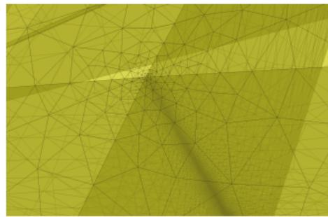
*enforced refinement at cracks*
