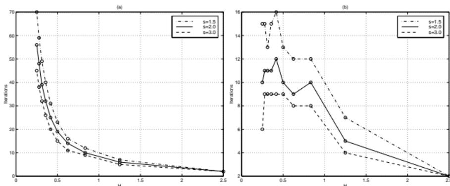
Iterations for  $H/h$  and  $H/\delta$  constant: (a) one level, (b) two levels.
