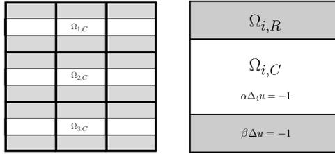
**Fig. 3** Left: Example for a decomposition of  $\Omega$  in  $N = 9$  subdomains, intersected by 3 channels  $\Omega_{i,C}, i = 1, 2, 3$ . We define  $\Omega_C = \bigcup_i \Omega_{i,C}$ . Right: Subdomain  $\Omega_i$  with channel  $\Omega_{i,C}$  of width  $\frac{H}{2}$ , where  $H$  is the size of a subdomain.
