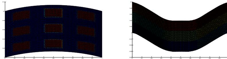
**Fig. 4** Left: Initial value (reference configuration) and two different materials with  $\nu = 0.3$  everywhere,  $E_1 = 210\,000$  in the red inclusions, and  $E_2 = 210$  in the blue matrix material. Right: Solution when a volume force  $f_v = [0, -10]^T$  is applied.
