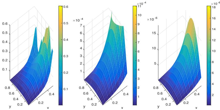
**Fig. 2:** Modulus of the error  $e_1^n := u - u_1^n$  for  $n = 1, 5, 15$  on the left subdomain when using the parallel Schwarz method for solving  $\Delta u - i\omega u = 0$ . Note how the modulus satisfies the maximum principle.
