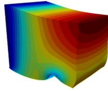
**Fig. 3:** Displacements of a clamped elastic cube over the sinus-shaped obstacle
