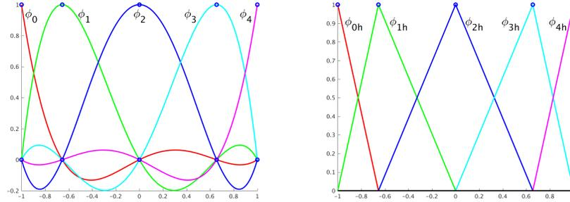
**Fig. 2:** One-dimensional higher-order (left) and linear (right) shape functions associated with GLL points for degree  $p = 4$ .
