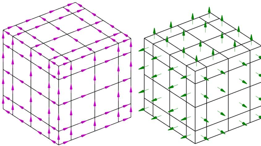
**Fig. 1:** Edge (left) and face (right) locations on three faces of a cube for a higher-order element of degree  $p = 4$ . Also shown is the corresponding assembly of  $p^3$  lowest-order elements on the associated Gauss-Lobatto-Legendre (GLL) mesh.
