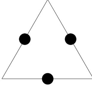
**Fig. 2:** The CR nodal points, i.e., the degrees of freedom of the Crouzeix-Raviart finite element space on a fine triangle.
