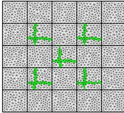
**Fig. 3:** The location of all jumps in  $\alpha(x)$ , where  $\Omega = [0, 1] \times [0, 1]$  is partitioned into  $5 \times 5$  subdomains. The values of jumps on the white and green triangles are 1 and 1.0e4, respectively. To get numerical results, we use these green channels as the periodic patterns for different number of subdomains.
