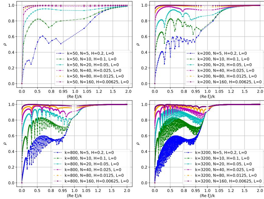
**Fig. 2:**  $\rho$  of Després' method for free space on  $[0, 1]^2$ .
