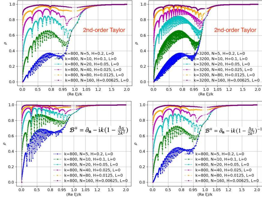
**Fig. 9:**  $\rho$  of Després' method plus a 2nd-order term for free space on  $[0, 1]^2$ .
