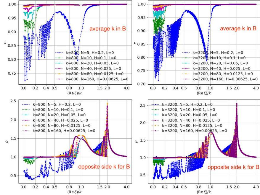
**Fig. 11:**  $\rho$  of Després' method on  $[0, 1]^2$  with exterior wavenumber  $k$  & interior  $k/[1, 5, 0.5, 2, 1]$ .
