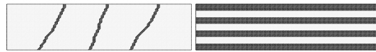
Fig. 1: Testcase 1 – partition ( N = 4 ) and distribution of E ( 10^8 if white and 10^3 if dark)
