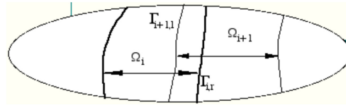
Fig. 5 Strip decomposition considered for substructured optimized Schwarz.
