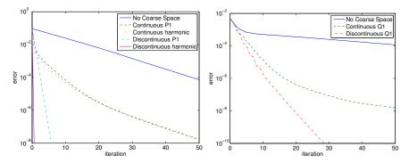
Fig. 1 Convergence curves of the DCS-DMNV algorithm in 1D (left) and 2D (right)
