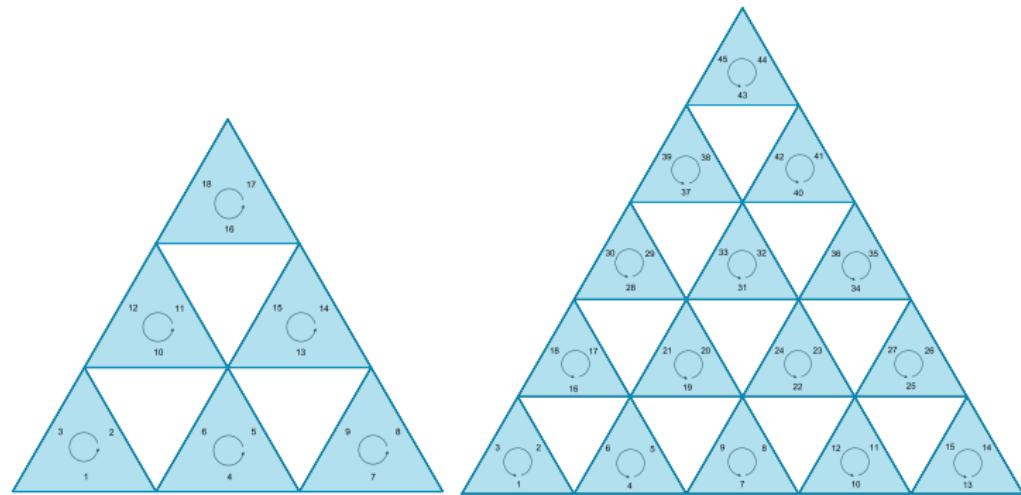
Dofs (and the corresponding basis functions) are associated with each **small edge** of each small triangle.
