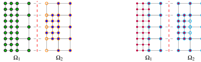
Fig. 3: An example of the classification of the degrees of freedom with Q_1 elements. Left: Subdomain \Omega_1 : ● locally owned dofs; ○ locally active dofs. Subdomain \Omega_2 : ● locally owned dofs; ○ locally active dofs. Right: Subdomain \Omega_1 : ● locally relevant dofs; Subdomain \Omega_2 : ○ locally relevant dofs.
