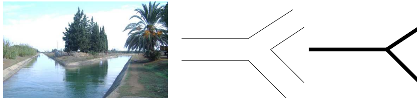
Fig. 1 Left: Irrigation channels in the vallée de la Medjerda, Tunisia. Middle: geometric shape of a junction. Right: simpler one dimensional approximation of the junction.
